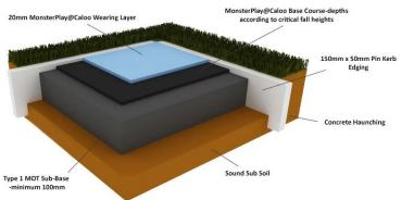
MonsterPlay@Caloo wet-pour surfacing is formulated from rubber granules and polyurethane binders. The surface consists of two layers: a base layer of coarse black granules made from recycled tyre rubber and a coloured top layer of much finer rubber granules.
