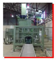
Challenger manufacture form, fill and seal machines for the automatic forming, filling and sealing of the plastic bale bags from a reel of film and will accommodate a variety of products including woodshavings, woodchip, copped straw, chopped hay and haylage.
