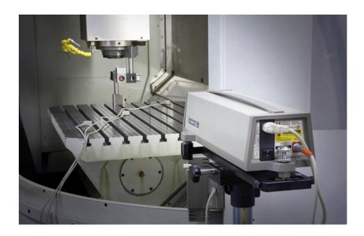
Our highly qualified Staff, together with Advanced Equipment and Computer Aided Technology, provide an unrivalled Machine Tool Measurement and Error Correction Service to machine tool users, suppliers and service companies. Our UKAS accreditation, with the lowest commercially available measurement uncertainty of  $0.15\mu m + 0.5\mu m/m$  for lengths up to 4m and  $1.9\mu m/m$  for axes up to 80m, gives the peace of mind of an internationally recognised certificate of machine performance.
