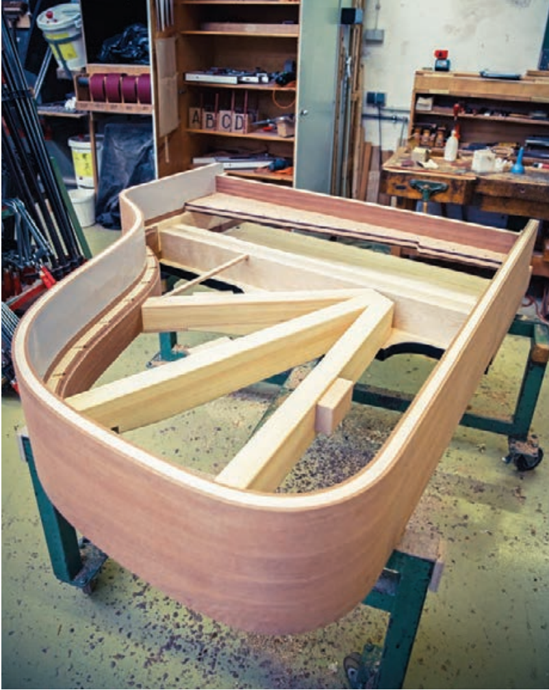
HERE: the piano rim is built up from some 20 thin, curved layers of wood, each with the grain running in the same direction, because it sounds better this way
