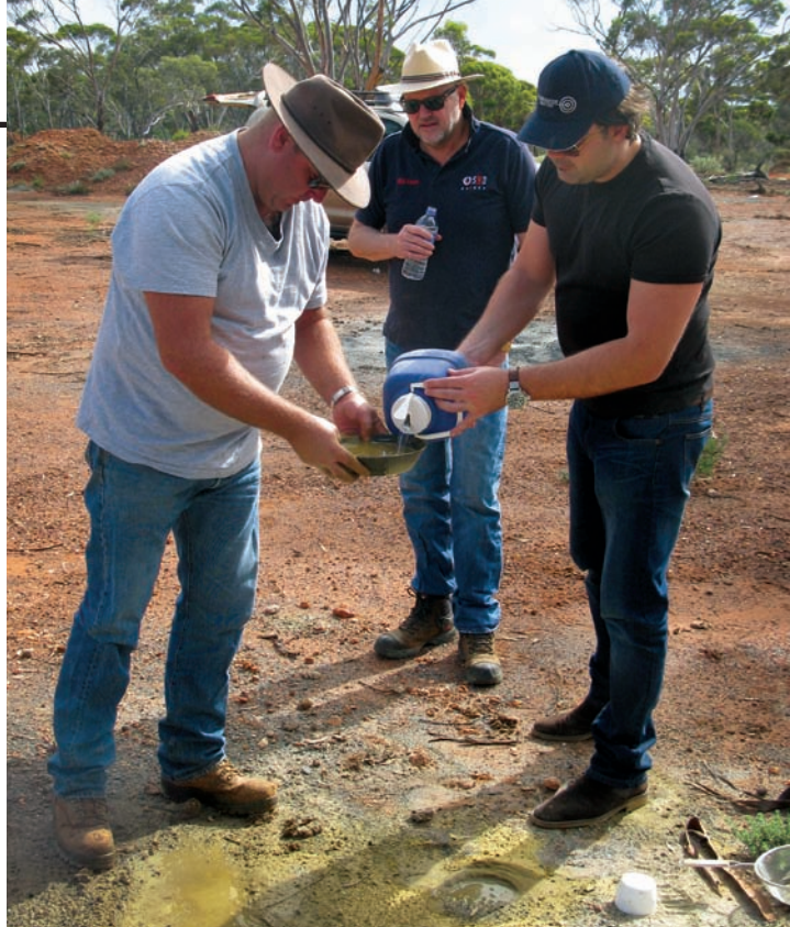
Panning drill intersections to confirm presence of gold for Golden Eagle Mining in Coolgardie.
