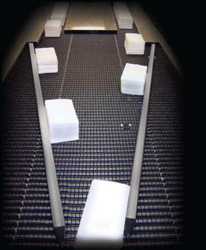
Sorting products from a single lane to multiple lanes for Tub Loading.
