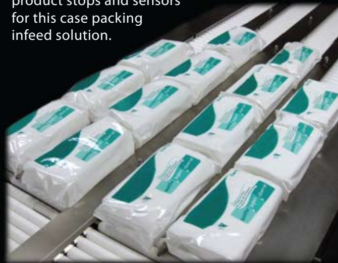
A variety of roller surface materials and 316 stainless steel construction is available
