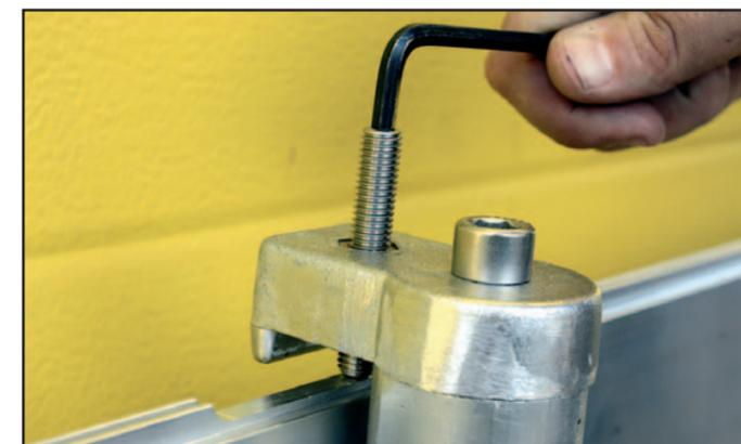
**4** On top of the compression post retainer, turn the 12mm cap screw, clockwise, by hand, until finger tight.
