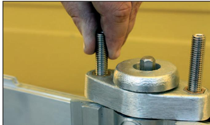
**6** On the front face of both the vertical side channels and the demountable posts, by hand, start turning the horizontal 10mm grub screws, clockwise, until they are finger tight.
