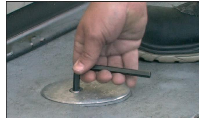
**4** Using the 10mm Allen Key, turn the 12mm cap screw anti-clockwise until the top compression block can be removed.
