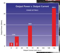
Indicative of the powers delivered by the Helica TC, the chart shows the low range at which the instrument works making it safer in comparison to other electro-surgical devices.
