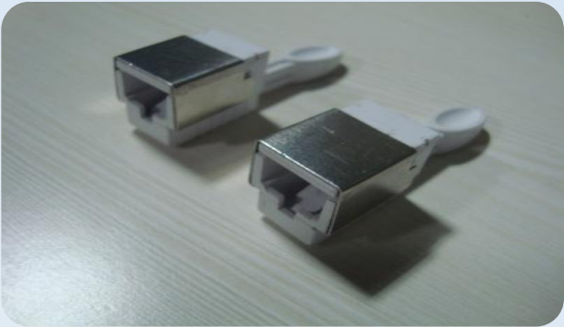
Patch chord lock.
