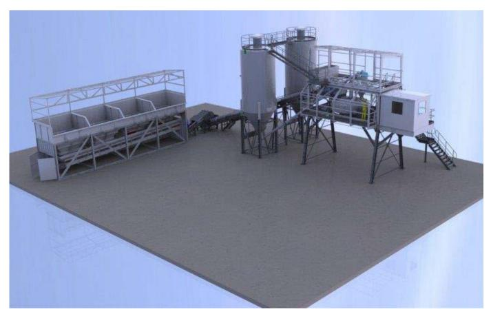
3D Drawing of our Semi-Mobile Batching Plant
