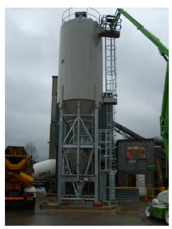
Vertical Cement Silo With Weigh Hopper
