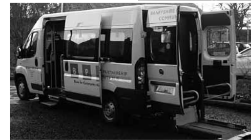
Left: Fiat Ducato - a clever combination of low floor and extra wide body, but in a lightweight shell, that enables it to be driven by those who do not have category 'D1' on their licence.
