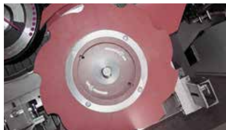
B & H's patented constant velocity starwheel system is standard on BH1600AB labelers.
