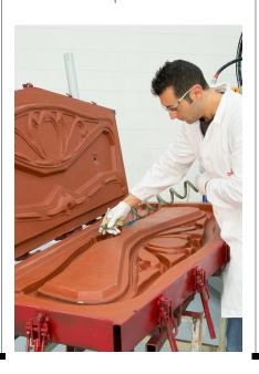
Polyurethane is spread into the mould with SAIP equipment.
