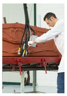
Polyurethane becomes hard and it's possible to open the mold. It takes the form of the mold.
