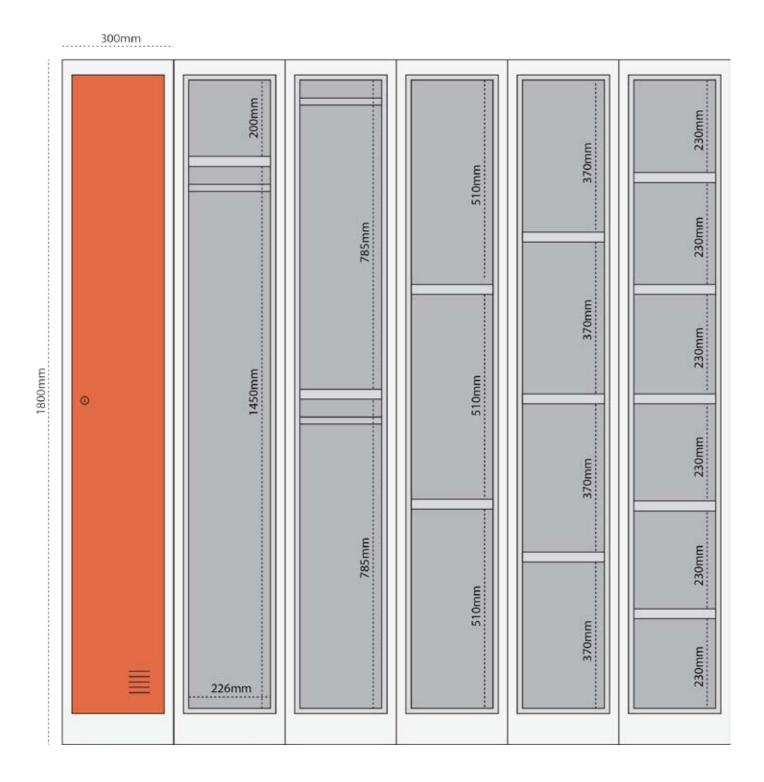
Interior dimensions shown above detail the size of the door opening, the actual internal space will be larger.
