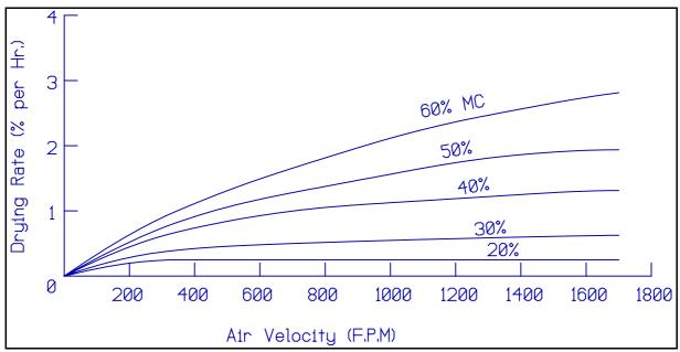
Figure 2 Combined Effect of Velocity and Humidity on Drying Rate
