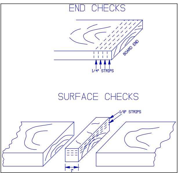
Figure 3 Checking for Checks
