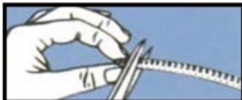
Step 1: Cut the center of the perforated holes in both the full and empty tape.
