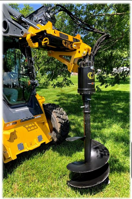
•Compact high torque planetary gearbox with Eaton motor
