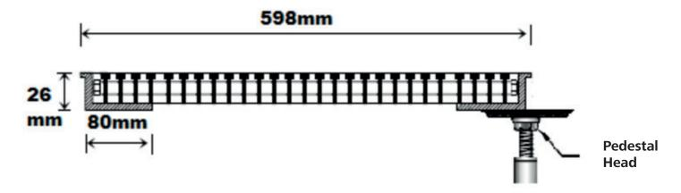
Computer room floor grille fitted with opposed blade damper (OBD)
