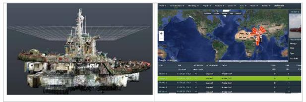
3) Digital Twinning (Digitalization) Vessel walkthrough using 3D scanning technologyto produce a 3D digital twin model for technical/operational support, and also marketing purposes. Links and embedded documents on key components in the 3D model allow viewers to navigate and monitor the important components of the vessel.
