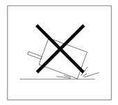
Handle the actuator carefully, do not drop it or subject it to excessive shock loading
