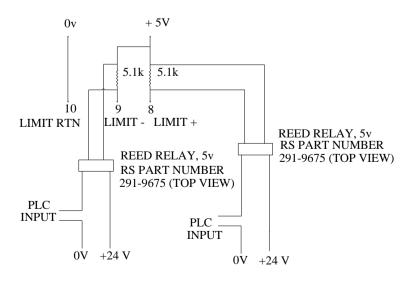
Limit Switch signal to 24V
