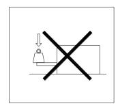
Do not apply excessive side loads to the rod, this can lead to increased friction and wear on the internal components
