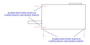
Fig 2. Actuator Mounting Points
