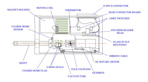
Fig 1. Actuator Components (LAR30-15 shown)
