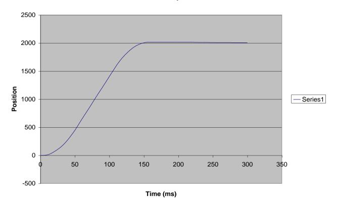
If this data is used to tune PID values, it can be seen from the graph there is a small amount of overshoot error at position. This can be eliminated by increasing the SI (set integral) or IL(integration limit) commands and running the profile again to verify.
