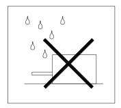
Avoid putting the actuator in hazardous environments such as wet, dusty, very hot (>50° C), very cold (<0° C). Consult SMAC if the actuator is required to work in these environments.
