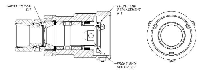
Emco Wheaton has developed a series of REPAIR KITS suitable for field repair of the J71 Series Couplers and Adapters.
