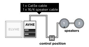
Each audio zone to be wired for multi-room audio will have a Cat5e + 4 core speaker cable run via a suitable control position (typically a switch level backbox), and then from the control position to the first speaker and then looped to the second speaker. This is the principle of the CEA/CEDIA 2030-A standard. Wiring in this way allows for the following options:
