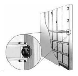
• Locate the top row of furring channel within 150mm of the ceiling.
