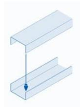
Screw the channel using Wickes Drywall Screws directly to a timber floor or drill, plug and screw using Wickes Nailable Plugs into a level concrete floor. The screws should penetrate the timber by at least 30mm. If a subfloor is particularly uneven it is recommended that a timber "sole plate" the width of the channel (52 or 72mm) and at least 30mm
