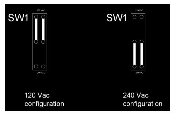
Figure 1. Control board SW1 jumper configurations for 120/240 Vac
