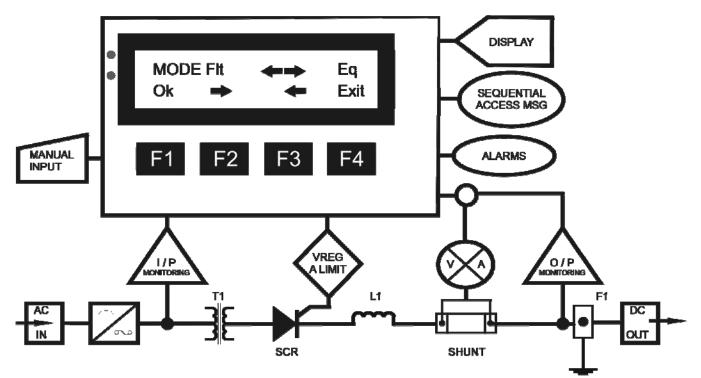
T1 : the AC supply is transformed and isolated.
