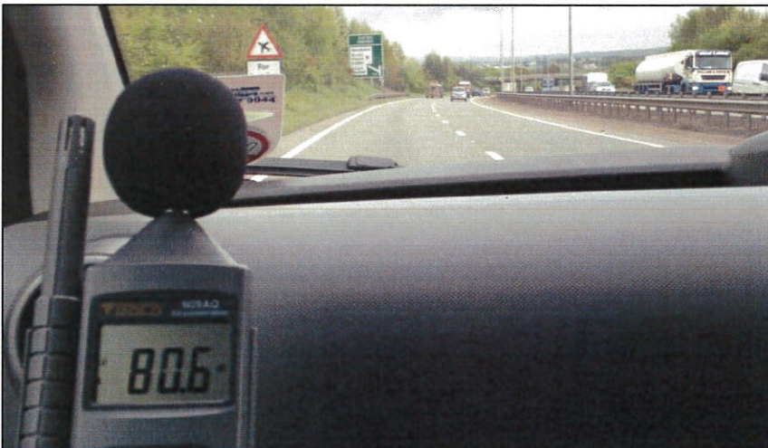
Noise reading taken with Ulti bars fitted.
