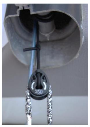
Tie the beam shockcord to the T2 single 29mm bock.
