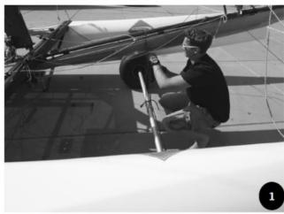
Tie the boat down on the Cat-Rack from the Spinnaker Pole
