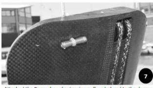
Attached the Daggerboard extension pull-up halyard to the daggerboard with a dog-bone to hold the daggerboard up from the ground.
