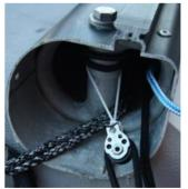
Lead the shockcord through the beam to the otherside, tie the 16mm harken block with the polyester rope to the beam casting to reverse the shockcord back the other entry side and tie on the shockcord to the beam casting.
