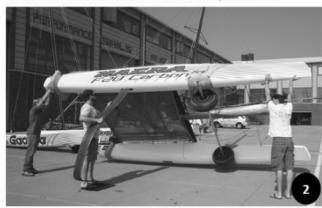
Insert the daggerboard with two or three persons. The figures below illustrates the preferable way to insert the daggerboards.
