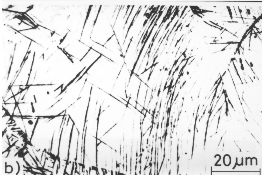
Fig. 8.8 Optical micrographs illustrating the microstructure of an ausformed bainitic steel: (a) alignment of sheaves of bainite in individual austenite grains; (b) curved bainite sheaves reflecting the deformation-induced misorientations within the austenite grains (Tsuzaki et al. , 1989).
