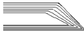
John Deere knife after cold forming : Continuous grain flow in the edges
