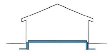
a. Band – shaped foundation use reinforced concrete or pre - fabricated materials with NBI Technical Approval.
