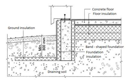
b. Band – shaped foundation use semi-continuous moulding of EPS, for example, Dorocell Byggsystem, Super Grund or analogic NBI Technical Approval materials.
