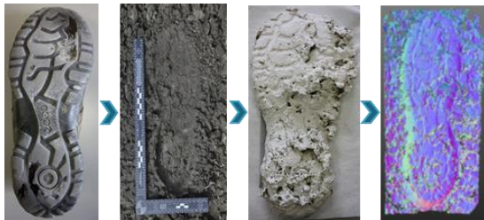
Fig. 9 Shoe, photograph, plaster cast and 3D data of impression in clay under field conditions. Comparison between the plaster cast and 3D data shows that the 3D data has more fine details that match with the original shoe.
