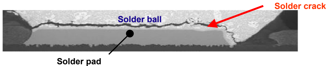
Figure #1: BGA interconnect with a printed circuit board failure:
