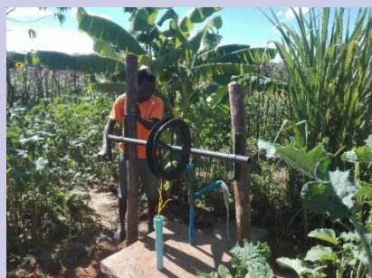
Above left: Rope and Washer hand pump Right: Self funded VIP latrine
