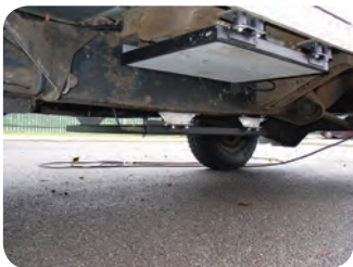
High power planar spiral antenna mounted under vehicle provide countermeasures
