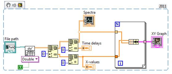
5. Next, we want to be able to baseline the spectra, which we notice are all offset from each other. We want to be able to select points on the spectra that we know should be zero, fit a line through those points, and subtract that line from the data. We will make vertical cursors to define the points. To do this, we go to the 'Cursors' tab of the XY graph properties and add a new cursor with the following parameters:
