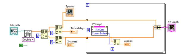
7. Next we want to read all the x-y position of all the cursors for each spectrum, fit a line through them, and subtract that line from the spectrum to re-baseline it. The following code achieves this, using the handy 'Linear Fit VI' from the mathematics tab:
