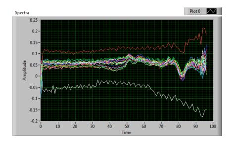
4. A more general way of displaying X-Y datasets is using an XY graph. The data-type of an XY graph is a 1D array of clusters, with each cluster composed of an array of the X and Y data respectively. This means we have to take each row of our data matrix, and 'bundle' it into a cluster with our x-axis labels. The following code achieves this:
