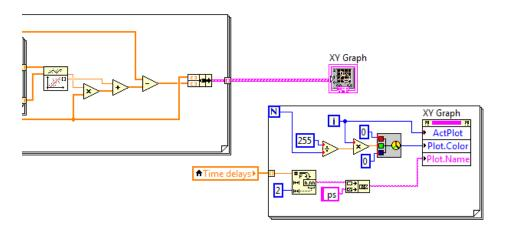
10. Remember that buffer '0' in the first cell of the input file we loaded earlier? We are now going to use that cell in the input file as a code for what units the X-axis is saved in. If it is a '0', the X-values in the file are in wavelength in nm, and if it is a '1' or anything else, we will assume the units are reciprocal centimeters. To do this, we will use a case structure. Case structures allow you only execute a certain block of code if a certain condition is met.
