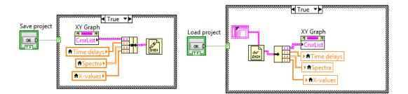
To load a binary file, you must input a cluster of the same format to the 'Read Binary File' VI so that it knows how to interpret the data it is reading. The easiest way to do this is simply to create a constant from the wire going
