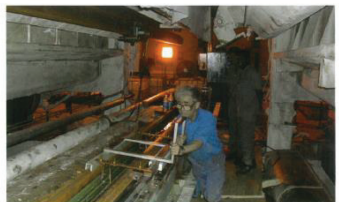
Electropolishing critical component surfaces at a paper making plant in India
