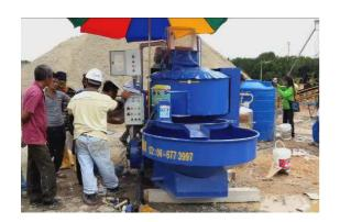
Cellular concrete is an ideal product for walls as it can be produced in a number of densities, each with its own properties. A higher density gives high strength, a lower density has higher insulation and fire rating properties. After mixing, cellular concrete is very liquid and fills the mould completely without vibrating.
