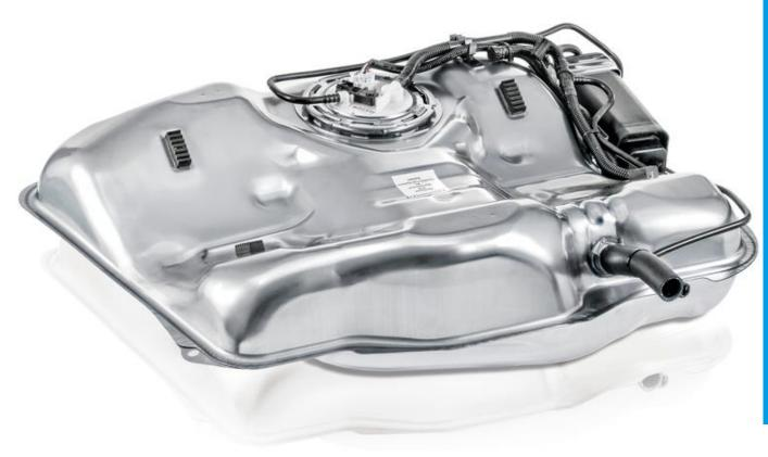
Use of Outokumpu HyTens® steel allows extremely thin walls and tailored strength, making the tank three kilograms lighter than the conventional fuel tank made of plastic
