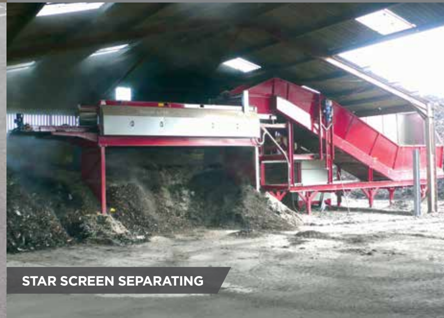
SINGLE EASYGRADE SCREEN MODULE
