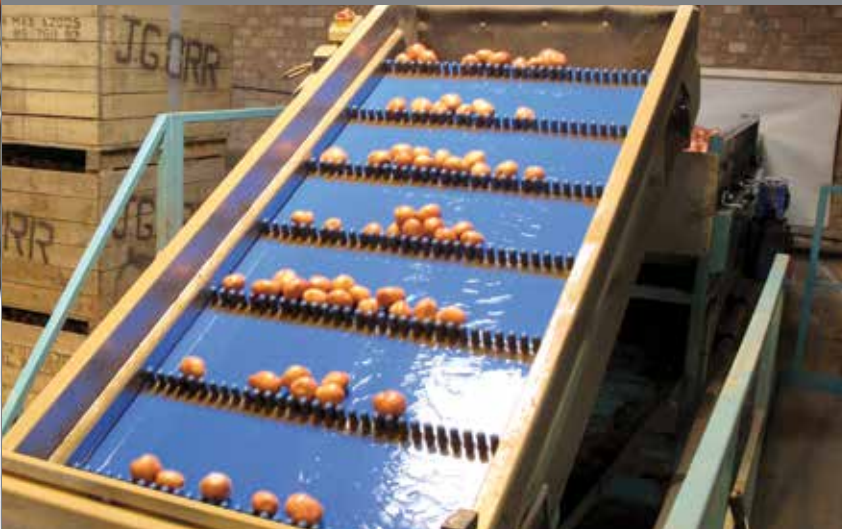
BARREL WASHER DISCHARGE ELEVATOR
