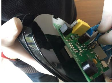
Step3: Disassemble the L (line, brown cable), N (neutural, blue cable) res1 and res2 (blue and red cable) sockets
