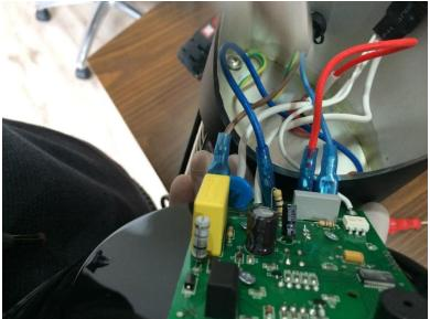
Step 13: Attach rezistance cables to res1 and res2 socket
