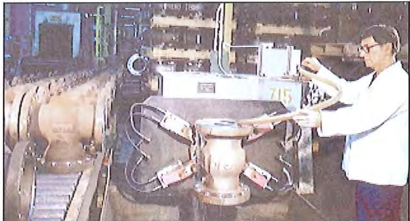
2 Air-under-water test of the seat's welds.
