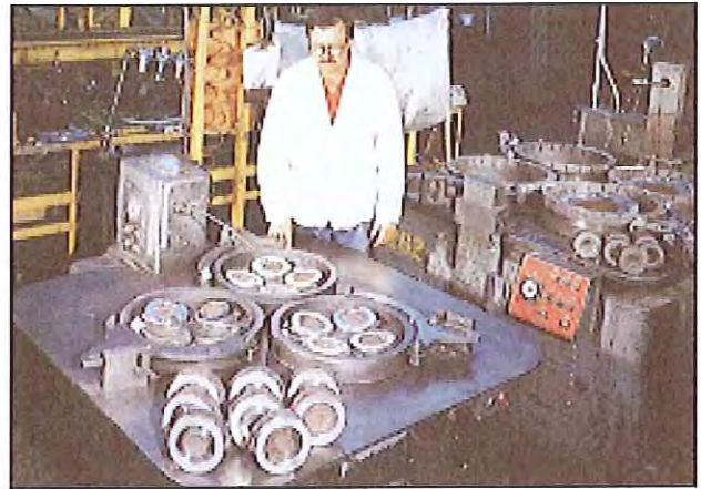
6 Lapping of wedge seating surfaces.
