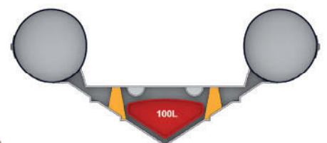
Hull sectional view with integrated fuel tank
