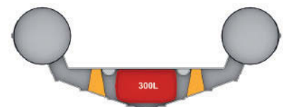
Hull sectional view with integrated fuel tank
