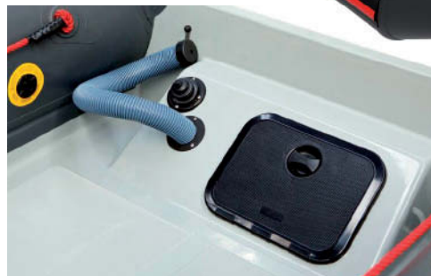
Bilge and pump access
