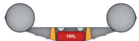
Hull sectional view with integrated fuel tank
