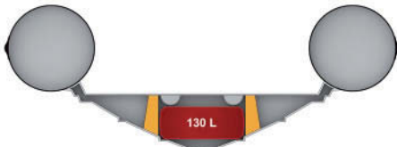
Hull sectional view with integrated fuel tank
