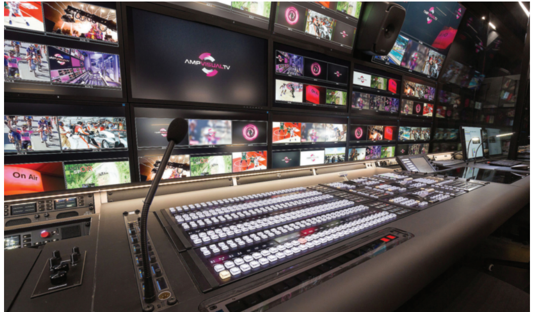
Millenium 6 is equipped with the Riedel MediorNet real-time media networking supporting as many as 26 wired and wireless cameras, a multiviewer monitor wall, and Artist (wired) and Bolero (wireless) intercom systems.
