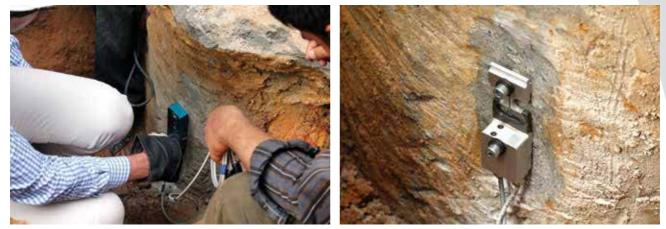
Fig 10. Preparation of combined acceleration and strain sensor
