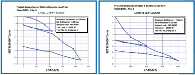
Fig 7. SLT of Pile#1
