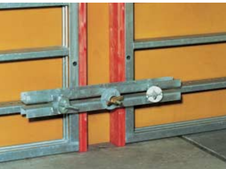
MANTO waler for length compensations of up to 30 cm and for the stopend. Can also be used with acute- and obtuse-angled corners.
