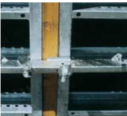
The adjustable aligning clamp is equipped with a sliding jaw, which permits a length compensation at the panel joint of 0-15 cm, independently of the grid holes.
