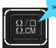
Measurements can be displayed on screen as mV, ohms/square or ohm.cm. There is a facility to input either probe spacing or wafer thickness so that ohm.cm values can be automatically calculated and displayed.
