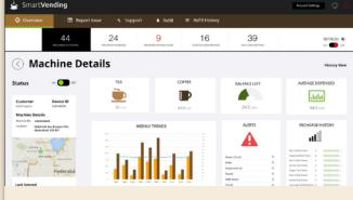
The web-based app provides significant detail on the health of the machine including alerts, recharge history and an ability switch on/off the vending machine. Further, iBot's client can remotely set the parameters of the machine so that the quality, quantity and temperature of dispensed coffee can be modified as appropriate to a region or customer profile.
