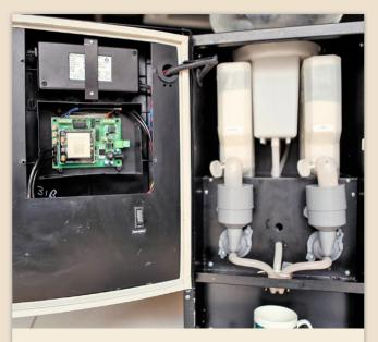
The assembly of Base Board + iQu Connected Processor are installed in the door of the vending machine, and the slot is closed so as to protect the entire assembly from the environment.
