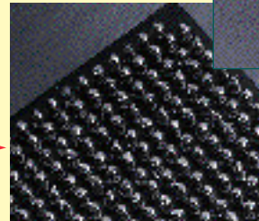
This surface mount module plugs into precision socket contacts built into the underside of the BGA carrier
