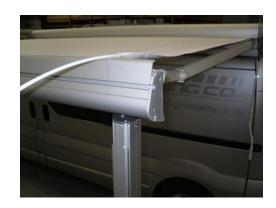
Take side awning rail section, these are square section aluminium bars with a flange either side, they are not handed. These can be supplied joined for storage purposes, make sure they are solid when fitting.
