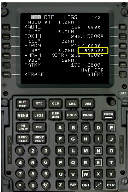
Fig. 17 “BYPASS” indication on CDU
