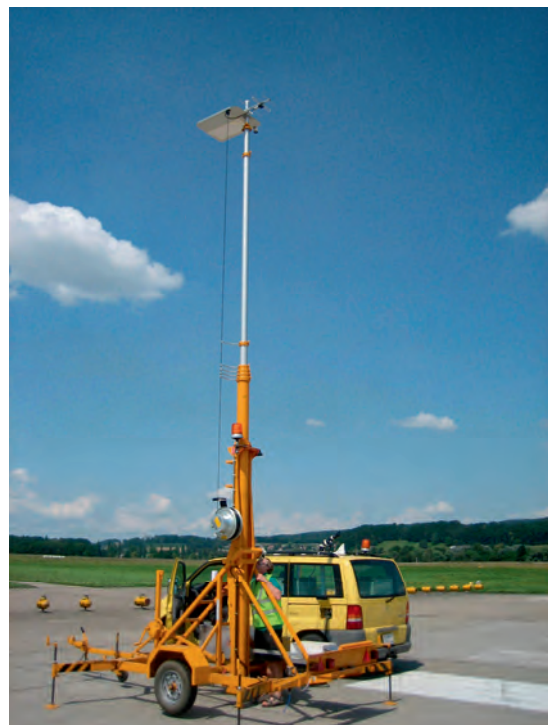
Figure 6. Telescopic Mast and Measurement Vehicle in the GP Mode Configuration
