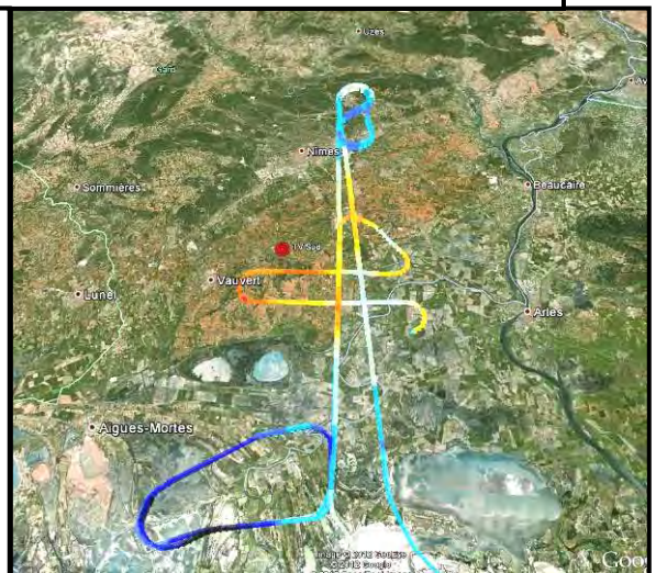
Flight Inspection trajectory. The color is function of the RFI field strength.
