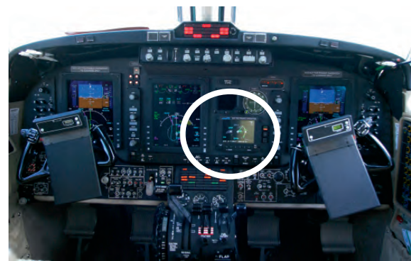
Figure 2: Cockpit of Flight Inspection Aircraft highlighting the Cockpit information Display
