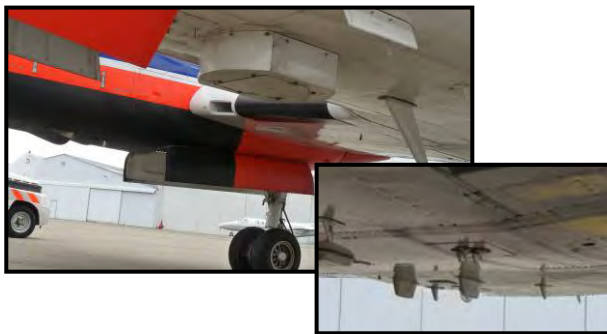
VHF/UHF DF and L band array below Be200
