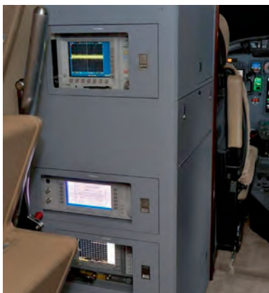
AFIS Equipment Cabinet
