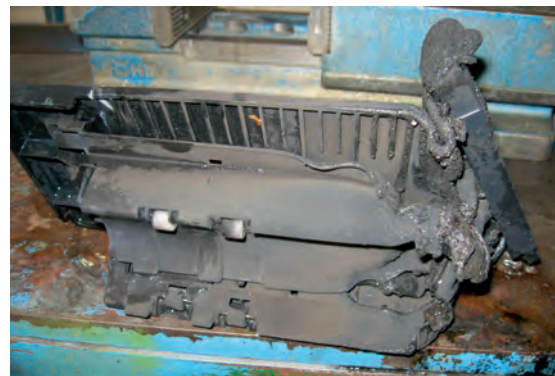
Printer cover after 60 seconds of fire
