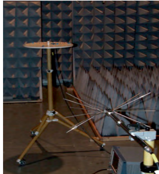
Figure 2: Antenna calibration in absorber chamber
