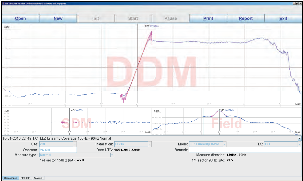
Figure 11. LOC Coverage: Correlation between Flight Check (in blue) and Ground Measurements (in pink)
