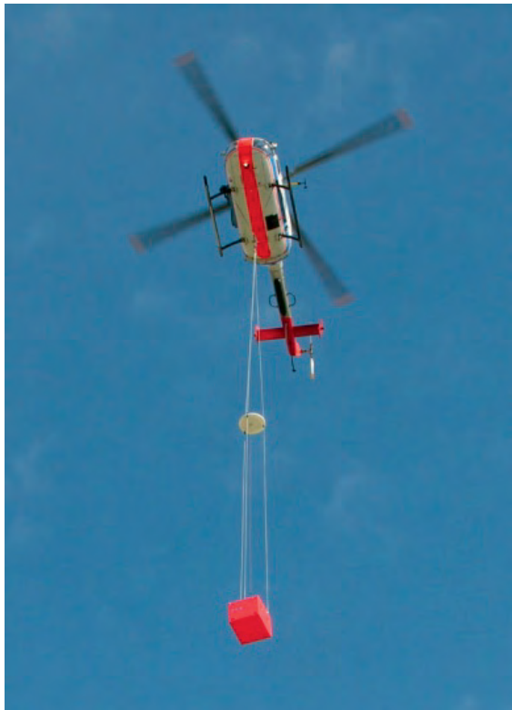
Figure 3: Helicopter carrying reference antenna
