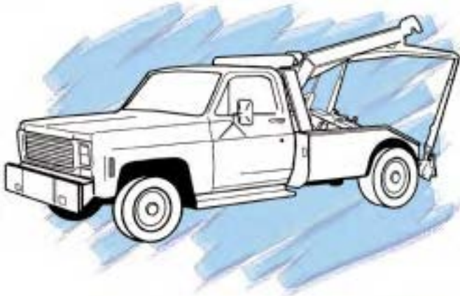
TOW TRUCK (Hydraulics raises boom)
