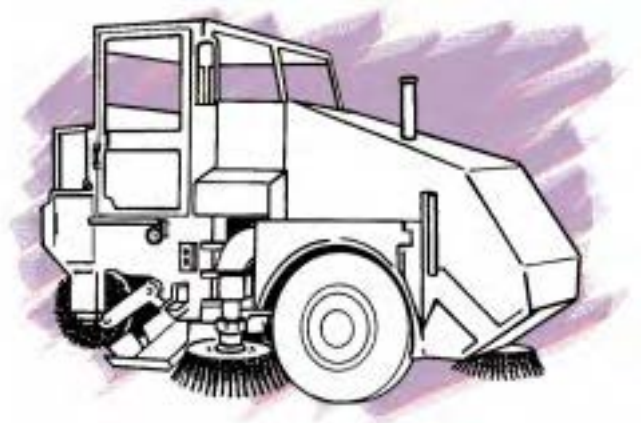
STREET SWEEPER (Clutch turns pump from engine)
