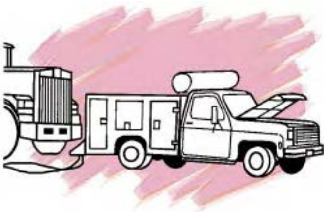
MOBILE SERVICE TRUCK (Clutch automatically turns on compressor when needed through relief valve/switch)
