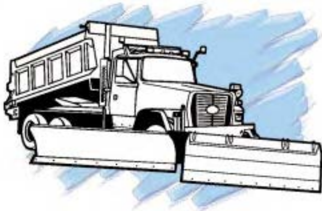
SNOW PLOW (Hydraulics raises blade)
